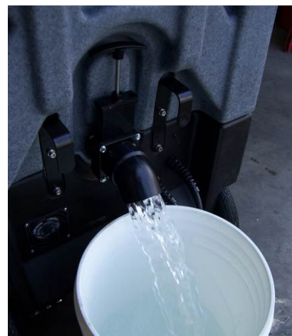
Drain water from Recovery Tank
